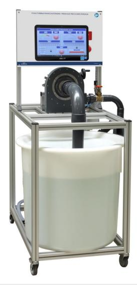
The TH 04.2 model is an advanced, scaled-down Francis turbine (or reaction turbine) simulator, specifically designed to facilitate detailed study and real-time visualization of the behavior and dynamic properties of such turbines.
